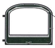
Replace the gasket by setting in place.
