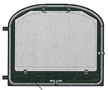
Un-screw the glass retaining screws and place Glass, Clips and Screws to one side.
