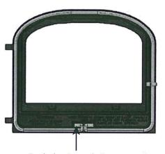
Push the Ceramic Rope firmly into place starting at one end. Take care not to stretch the rope during this process.
