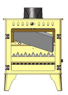
Lift the Baffle Brick and slide to the left. When the right side of the Brick clears the Baffle Support, lower the Brick into the Fire Box and remove.
