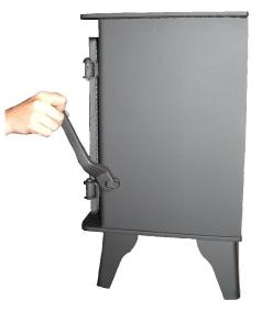
**To burn wood**, push the operating tool up and away from you. When left in this position, air is restricted through the bed of the fire providing a solid base to build up a bed of ash. Surplus ash can be removed either by gentle riddling or with a shovel.
