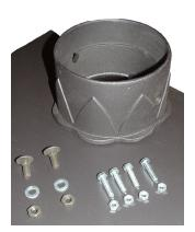
Place the Flue Gasket on the top, or rear outlet as required. Place the Flue Collar on top of the Gasket. Secure to the four locating tabs, inside the flue outlet, using the M6 nuts & bolts supplied. Fit the 2 - M8 carriage bolts, washers & nuts into the Damper Holes, located on each side of the Flue Collar.
