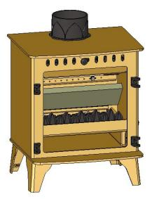
Pull the top edge of the Rear Brick forward and lift out of the Stove.
