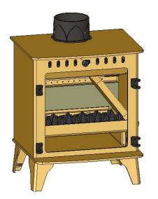
Pull the top edge of the Side Brick into the centre of the Stove, whilst lifting it out of the Side Plate
