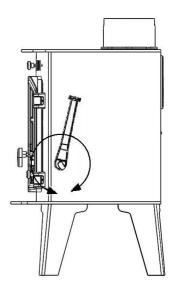
The ashpan should be emptied at least daily and ash should never be allowed to build up over a period of time as this will result in damage to the fire bars. The flat end of the riddling tool can be used to carry the ashpan.
